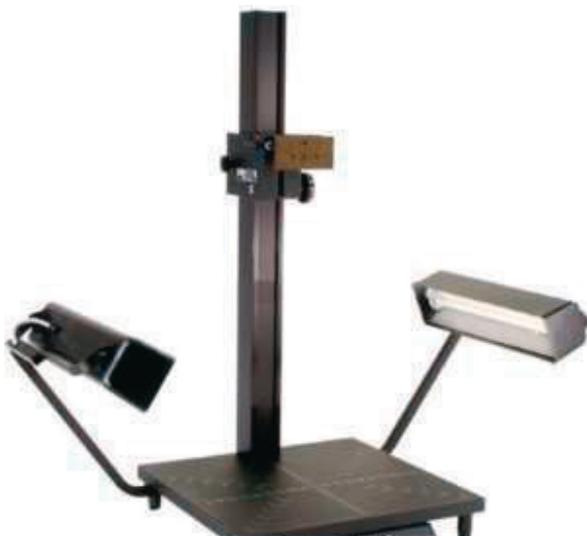
*copy stand with adjustable camera and lamp positions*
