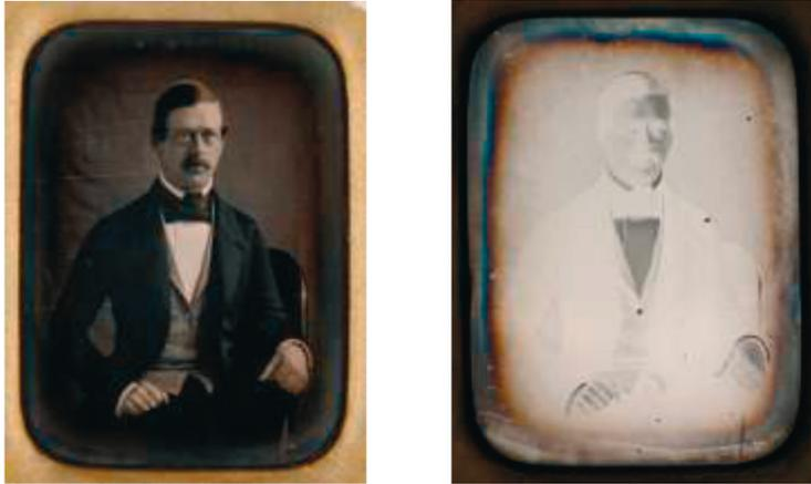
*standard frontal illumination (45° from left and right) and specular illumination (using sheet of glass at 45° between camera and object)*
